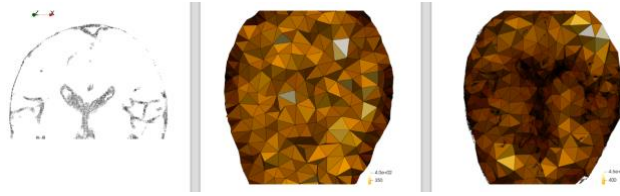
Figure 15. Registration points (left), isotropic mesh (center) and anisotropic sub-optimal mesh (right).
