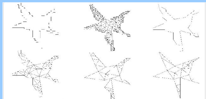
(Top Left) Original image. (Top Middle) Triangulation of original image. (Top Right) Image after line-simplification with tolerance 1.0 (Bottom Left) Triangulation. (Bottom Middle) Triangulation of image with tolerance level of 2.0. (Bottom Right) Triangulation of image, tolerance of 3.0.
