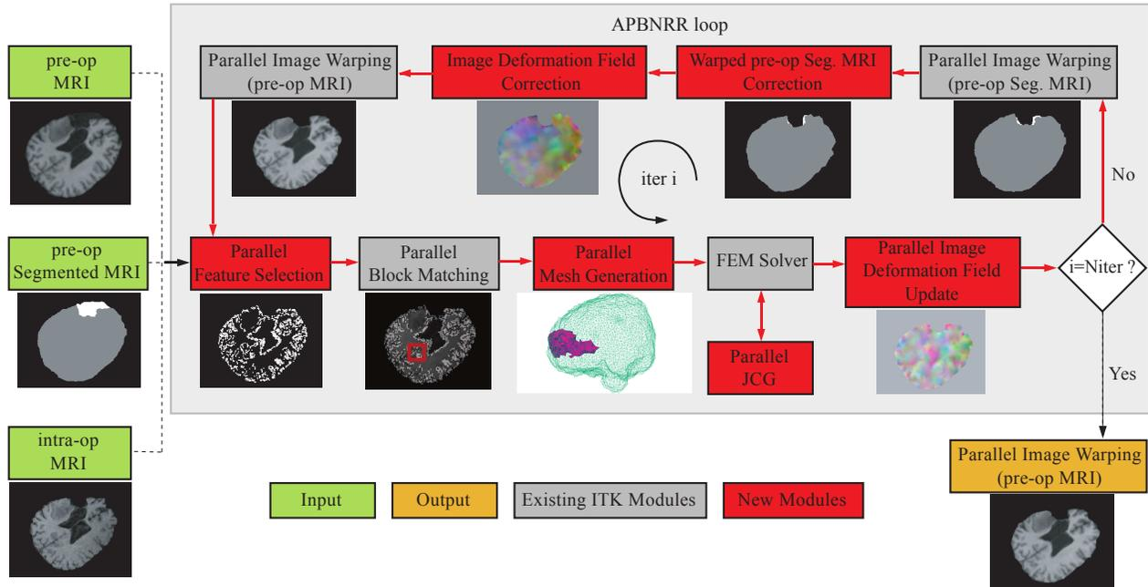
**Figure 1.** The APBNRR framework [6]. The green, red and gray boxes represent the input, the new contributions and the existing ITK modules, respectively. The red arrows show the execution order of the modules. Orange represents the output warped pre-operative MRI.
